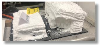
Photograph 1: Intumescent char expansion unrestricted during testing.
