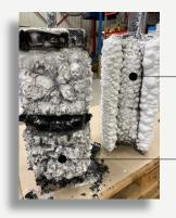
Structural steel **Column 01** (reference column) after fire testing.
