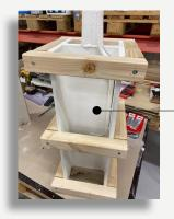
Structural steel **Column 02** prior to fire testing clad with 50X50mm timber strapping.
