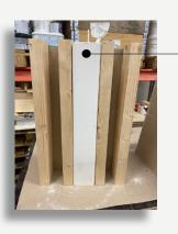
Structural steel **Column** 02 prior to fire testing clad with 90X45mm timber framing and plasterboard hard against the steel face.
