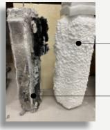
Structural steel **Column 01** (reference column) after fire testing.
